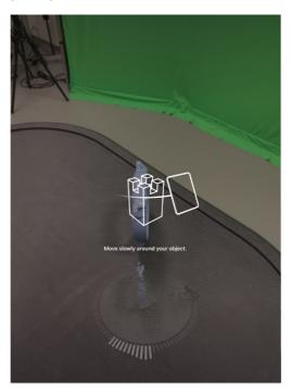
Subsequently the AI in the app creates the 3D Model. The 3D model is saved as in the usdz-format. By using an online file converter the file is converted into a .stl-file, which can be read by e.g. the free CAD program Blender.
